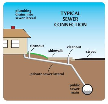
A private sewer lateral (PSL) is the pipe that connects the plumbing in a home or business to the sanitary sewer main, usually located in the street. The PSL carries sewage from a building to a public sanitary sewer. It is the responsibility of the property owner to maintain the sewer lateral.
